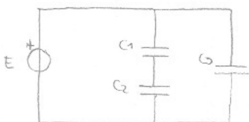
$$\frac{1}{C_{TOT}} = \frac{\left(\frac{1}{C_1} + \frac{1}{C_2}\right) \cdot \frac{1}{C_3}}{\frac{1}{C_1} + \frac{1}{C_2} + \frac{1}{C_3}}$$
